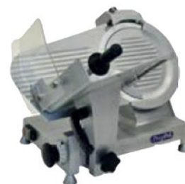
Compact Slicer, manual, gravity feed, 12" diameter knife, up to 9/16" slice thickness, built-in sharpener, permanent ring guard, knife cover interlock, sealed splash zones, square receiving plate, on/off power switch, overload protection, 1/3 HP, 120v. Item # 18105 & 17061 ATOSA Mfg. # PPSL-10 & PPSL-12 Ea
