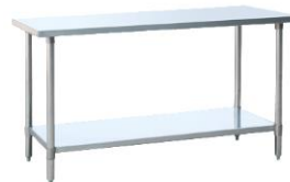
Work Table, 24"W x 24"D x 34"H, 18 gauge stainless steel top with turned down edges, adjustable galvanized undershelf, galvanized legs, and adjustable bullet feet. Item # 10026 Atosa Mfg. # SSTW-2424 Ea
