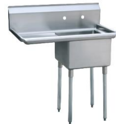
One compartment sink, 39"W x 24"D x 44-1/2"H overall, (1) 18"W x 18" front-to-back x 12" deep sink compartment, 18" left hand drainboard, 18 gauge stainless steel, galvanized legs. Item # 21112 Atosa Mfg. # MRSA-1-L Ea
