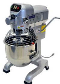
Planetary Mixer, 21 & 32 quart capacity, floor model, #12 hub, gear driven, (3) speed controls, side mounted controls, 30-minute timer, includes: stainless steel bowl & guard, wire whip, aluminum flat beater & dough hook, 1-1/2 HP, 1100 watts, 14 amps, 115v. Item # 20581 & 20580 ATOSA Mfg. # PPM-20 & PPM-30 Ea
