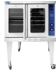
Convection Oven, gas, single-deck, 50/50 dependent doors with double pan thermal tempered glass, 150 to 500F temperature range, digital controller, 2-speed-fan with adjustable cool down mode, interior lighting, 5 wire racks. Item # 20363 ATOSA Mfg. # ATCO-513B-1 Ea
